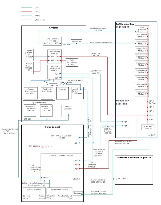
Figure C-1. DynaCool System Interconnects for 9 T System
