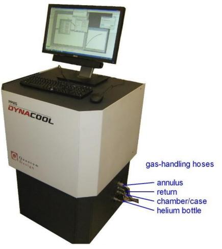
Figure 2-5. Front view of Pump Cabinet.
