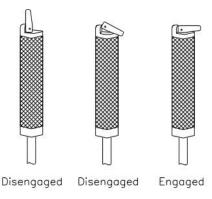
Figure 1-4. Operation of puck insertion tool.
