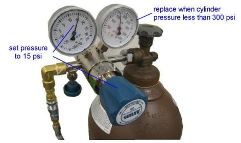
Figure 2-9 Helium gas bottle with regulator.
