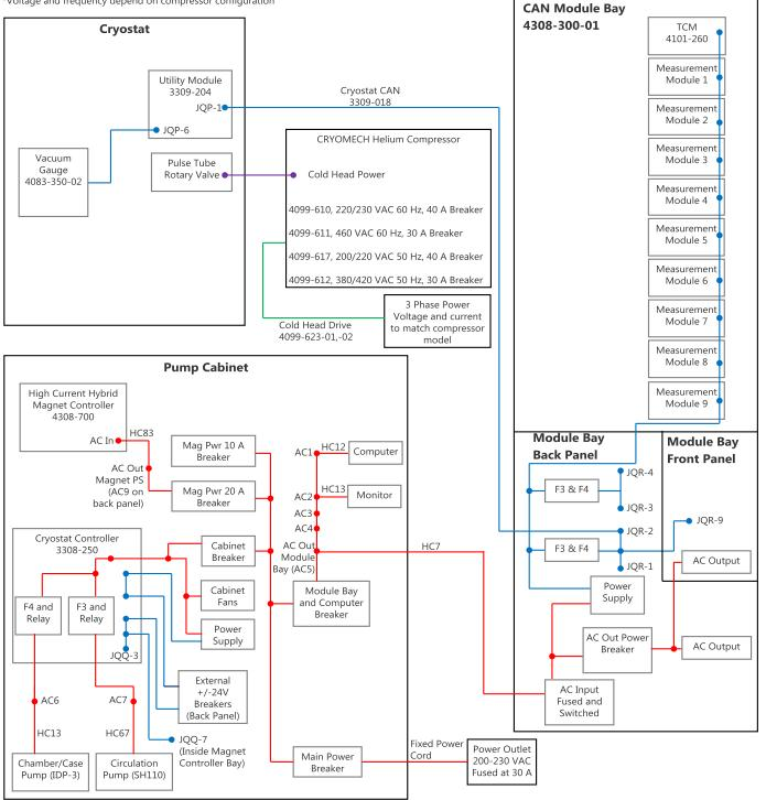
Figure C-4. DynaCool Power Distribution for 14 T System
