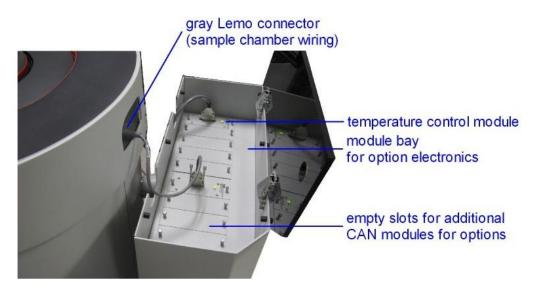
Figure 2-3. CAN Module Bay and sample puck wiring port (gray Lemo).
