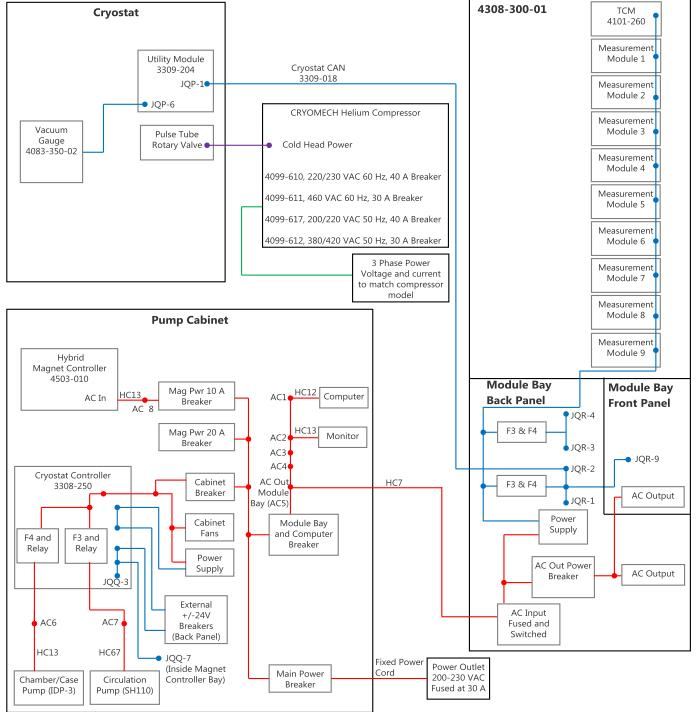
Figure C-3. DynaCool Power Distribution for 9 T System
